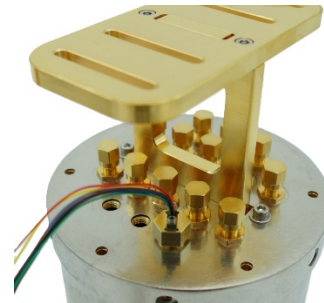
(Optional) 9-pin nanoD DC feed-thru (top view)
