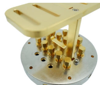
16x 1/4-36 threaded feed-thru
