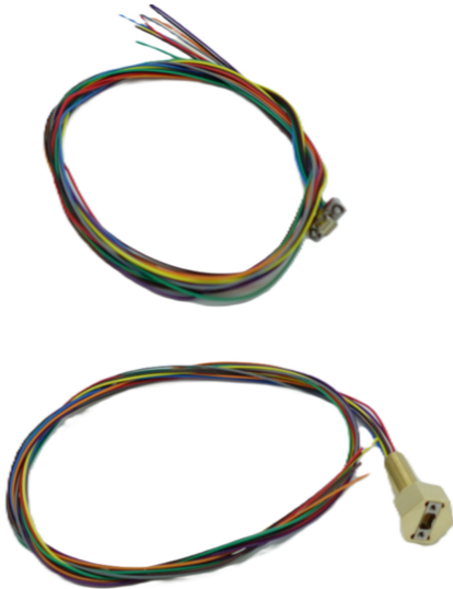
(Optional) 9-pin Omnetics nanoD DC feed-thru
