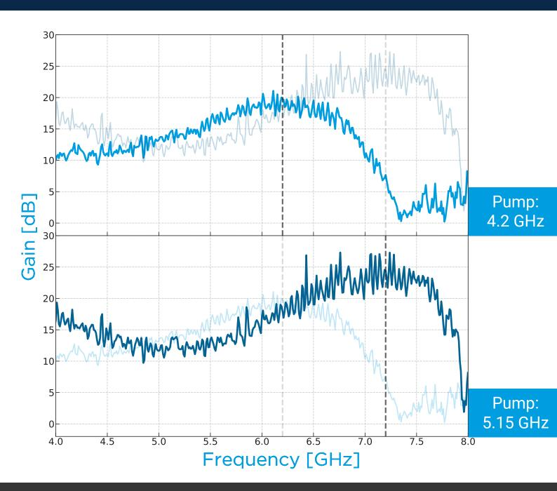
The above plots show the gain profile of a single device measured for two different pump frequencies. By tuning the pump, one can measure devices in the 4-8 GHz band within a single cooldown.
