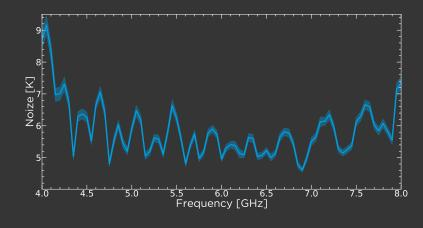
Typical noise of the setup used to characterize the devices (WITHOUT TWPA, HEMT ONLY).
