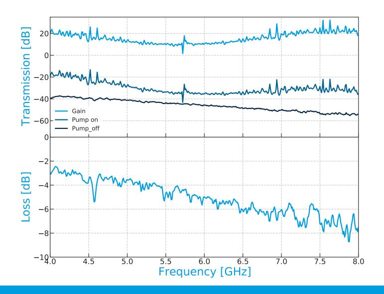
To achieve high-gain over a band exceeding 3 GHz, phase-matching between the pump, the signal and the idler is required.
