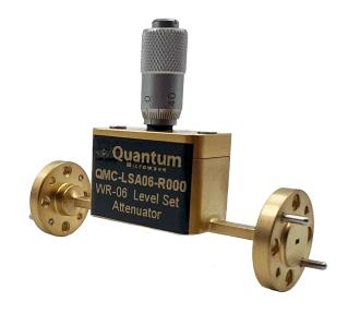
QMC-LSA06-R000 is a D Band Level Set Attenuator and covers a frequency range of 110 to 170 GHz. This attenuator is equipped with a micrometer dial. This attenuator is ideal for a waveguide system where broadband level setting is required.
