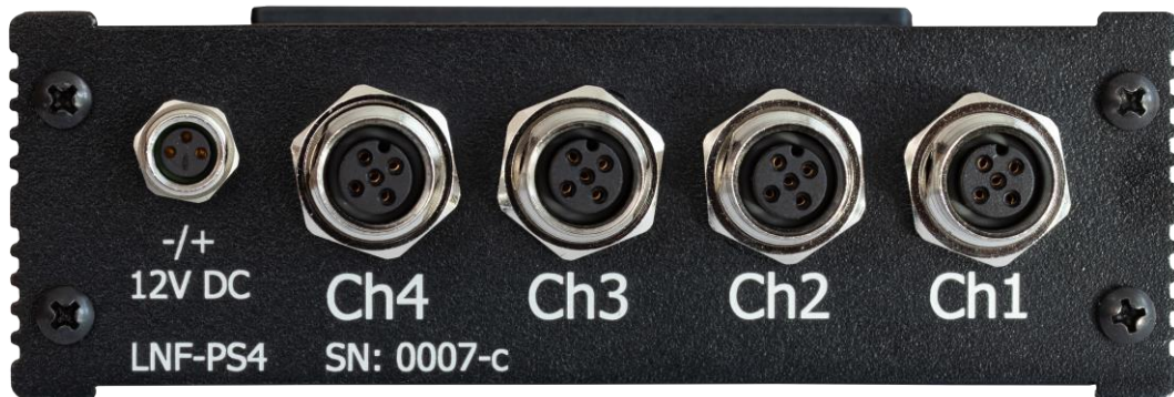
Figure 2 Rear panel equipped with four female socket 5p connectors size M12.
