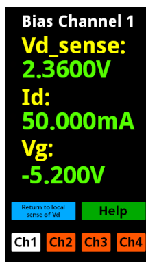
Figure 8 Screen when LNF-PS4 in remote sense mode
