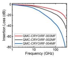
Insertion loss above 40 GHz is estimated from ECCOSORB® absorption measurements:
