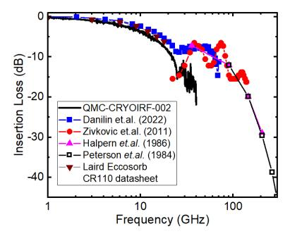
Insertion loss of QMC-CRYOIRF-002 filter (solid black line) plotted with insertion loss data derived from measured absorption of Eccosorb CR110 from literature [1-4] scaled to the dimensions of the QMC-CRYOIRF-002 filter. Above 300 GHz the absorption coefficient is expected to continue to vary with frequency as a power law [3].
