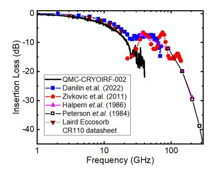
Insertion loss of QMC-CRYOIRF-002-S filter (solid black line) plotted with insertion loss data derived from measured absorption of Eccosorb CR110 from literature [1-4] scaled to the dimensions of the QMC-CRYOIRF-002-S filter. Above 300 GHz the absorption coefficient is expected to continue to vary with frequency as a power law [3].
