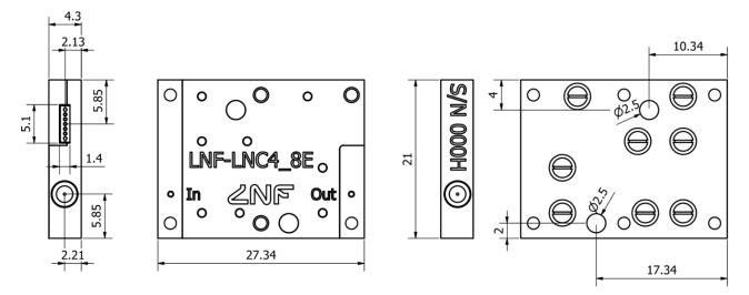
5-pin strip connector seen from outside the LNA (engraved text upward)
