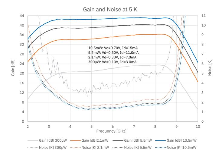
\* Test report submitted with each delivered LNA might vary slightly from this datasheet due to the G3PO to SMA adaptors used in our test systems not being corrected for.
