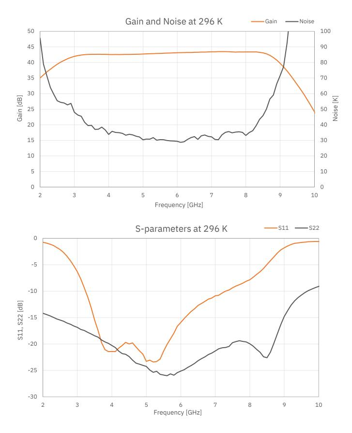
Nellickevägen 24, 412 63 Göteborg, Sweden info@lownoisefactory.com lownoisefactory.com Date 2022-03-28 **Datasheet** LNF-LNC4\_8E 4-8 GHz Cryogenic Low Noise Amplifier
