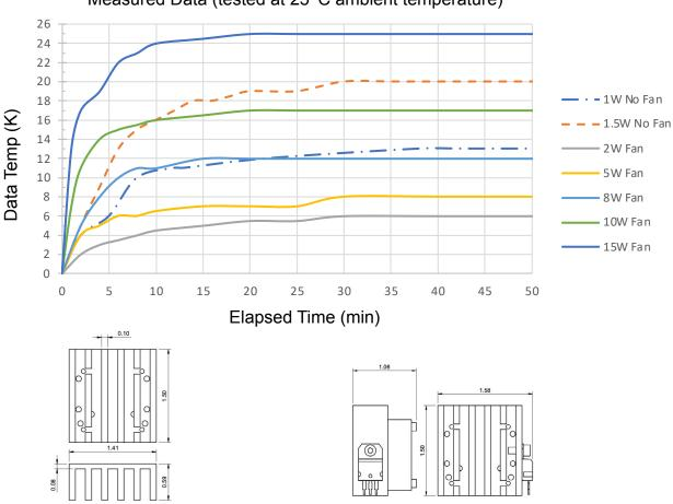
Measured Data (tested at 25° C ambient temperature)
