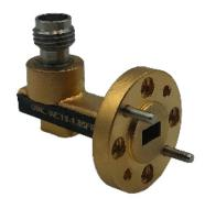
QMC-WC19-1.85FR385 is a Waveguide to Female Coaxial adapter that operates within the U Band, with a frequency range of 40 to 60 GHz. This adapter is a WR-19 waveguide with precision tolerances. QMC-WC19-1.85FR385 is a gold plated, copper waveguide with brass flanges. This is a lab asset that will last for long periods of time.
