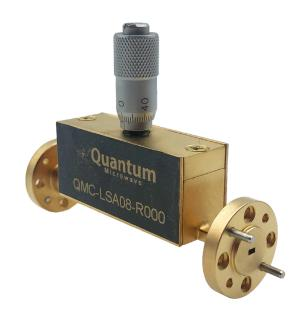
QMC-LSA08-R000 is a F Band Level Set Attenuator and covers a frequency range of 90 to 140 GHz. This attenuator is equipped with a micrometer dial. This attenuator is ideal for a waveguide system where broadband level setting is required.
