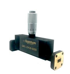
QMC-LSA28-S000 is a Ka Band Level Set Attenuator and covers a frequency range of 26.5 to 40 GHz. This attenuator is equipped with a micrometer dial. Our attenuator is ideal for a waveguide system where broadband level setting is required.
