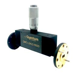
QMC-LSA22-R000 is a Q Band Level Set Attenuator and covers a frequency range of 33 to 50 GHz. This attenuator is equipped with a micrometer dial. Our attenuator is ideal for a waveguide system where broadband level setting is required.
