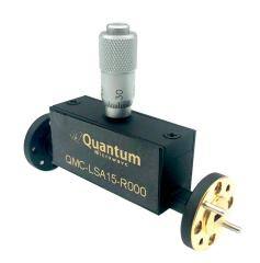
QMC-LSA15-R000 is a V Band Level Set Attenuator and covers a frequency range of 50 to 75 GHz. This attenuator is equipped with a micrometer dial. Our attenuator is ideal for a waveguide system where broadband level setting is required.
