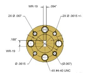
Comes with quantity 4 pcs of 4-40 captive waveguide screws Made in the USA
